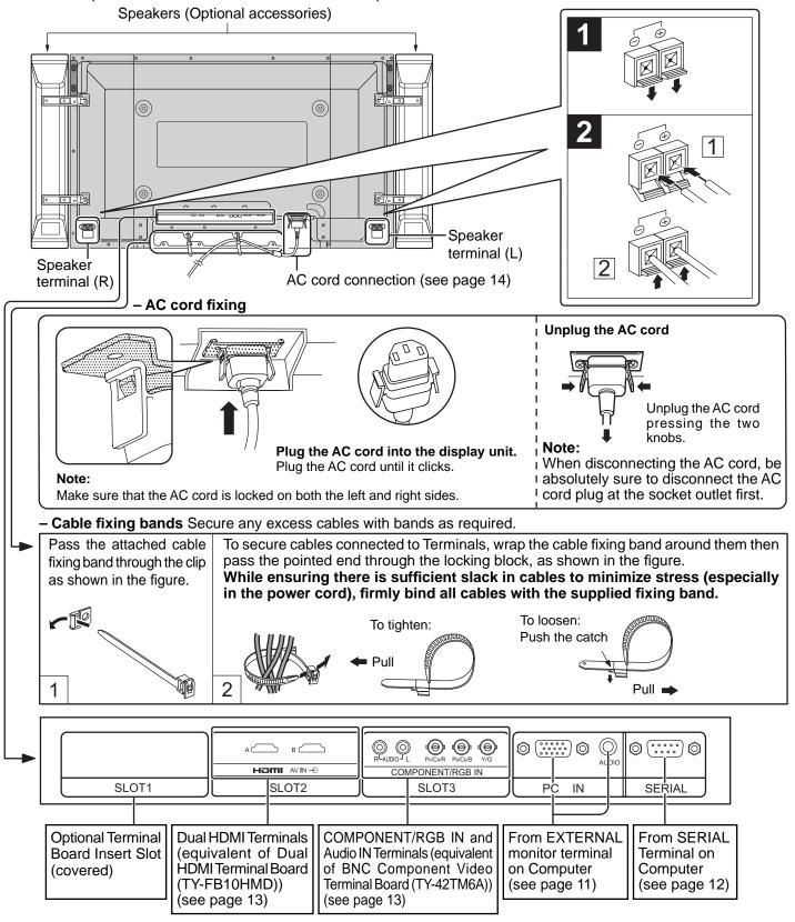
Note: At factory shipment, Terminal boards are installed in SLOT 2 and SLOT 3.
